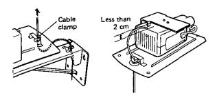
Attach the solid state color camera to the mounting angle on the bottom plate using with supplied bolt and washer.
