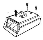
Attach the bottom plate to the housing mounting bracket using with supplied four screws and washers.
